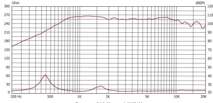
Frequency (Hz), Measured-1W@1M
